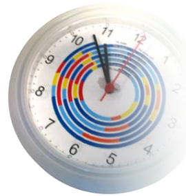
Figure 5.2: MarkerClock: Initial design. Each clock displays the activity of the home in which its paired clock is placed.
