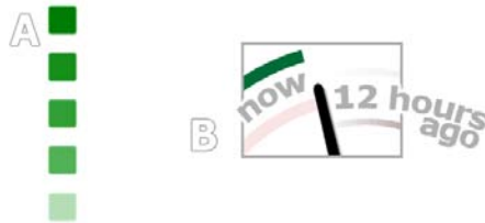
Figure 5.3: MarkerClock: A. Coding of the motion values as different transparency values, B. Fading of the trace at the last hour, as well as a unsaturation of colors in the last six hours of history.
